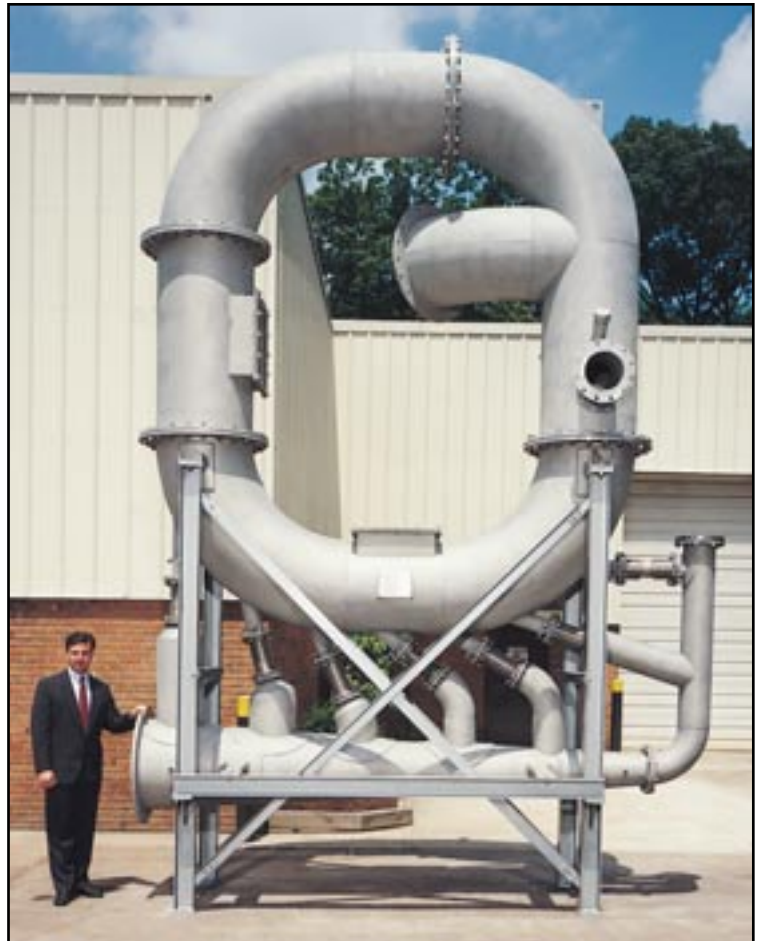
The Model 26 ThermoJet was designed to dry zeolite filter cake from an initial moisture content of 40% to a final moisture content of 10%, at a rate of 8000 lbs./hr.
